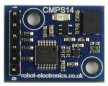
For **I2C** the mode pin can be left open or pulled to the supply voltage, for **serial mode** the mode pin should be connected to 0v ground.
